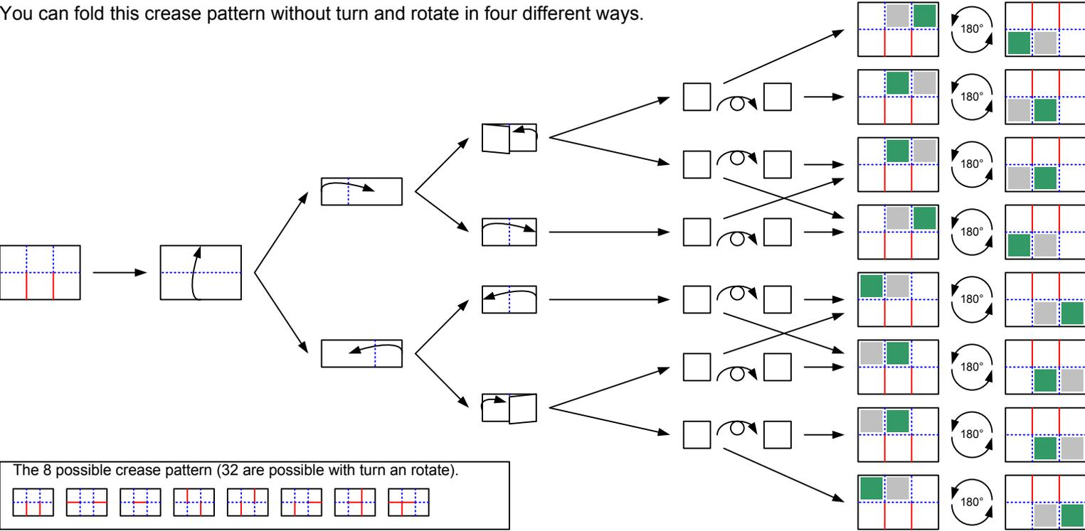
The 8 possible crease pattern (32 are possible with turn an rotate).
